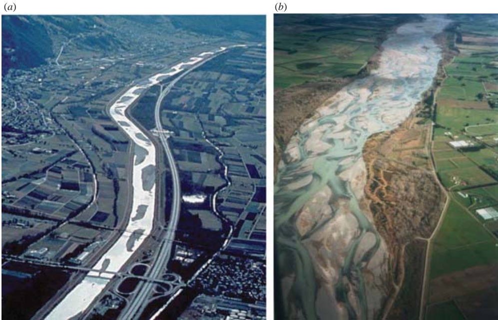
FIGURE 5. Free bars: (a) alternate bars in the Rhine River, Switzerland (Jaeggi 1984); (b) multiple row bars in the Waimakariri (braided) River, New Zealand (courtesy of B. Federici).
