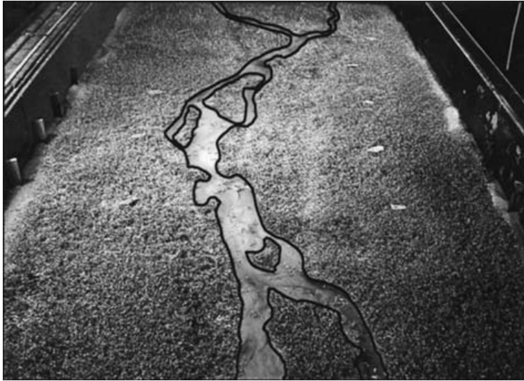
FIGURE 9. The laboratory experiment of Gran & Paola (2001): in the run with the highest spatial vegetation density the river resembled a wandering stream, with one to two main channels separated by large, vegetated islands.
