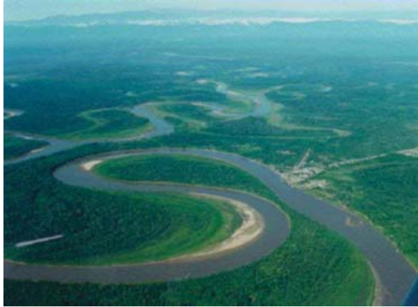
FIGURE 11. A meander bend close to neck cutoff showing that river width is a function of curvature and stage.
